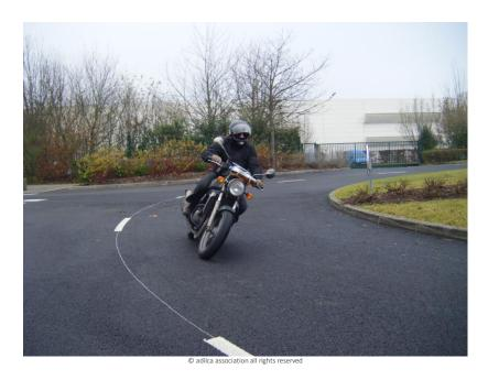
The experiment called 'water bottle' can reveal the true nature of the description. In dynamics, the liquid surface remains perpendicular to the motorcycle's plane of symmetry. In statics, the liquid falls on the side where the machine leans.
