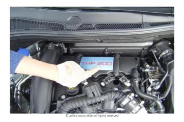
The power must be assessed in terms of the mass of the car, here 200 hp and 1,160 kg, a weight / power ratio equal to 5.8 kg / hp; to benefit from a favorable ratio, a 1,800 kg mass car should be equipped with a 310 hp engine.
