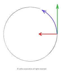
Device seen from above: the ball describes a circular path (blue arrow) because of the horizontal force (red arrow) transmitted by the string (axis and string do not appear in the drawing). If this force suddenly stops acting, for example in the event of a string breakage, the ball escapes by a rectilinear way (green arrow). There is neither centripetal force nor centrifugal force. Never add force, speed and trajectory!
